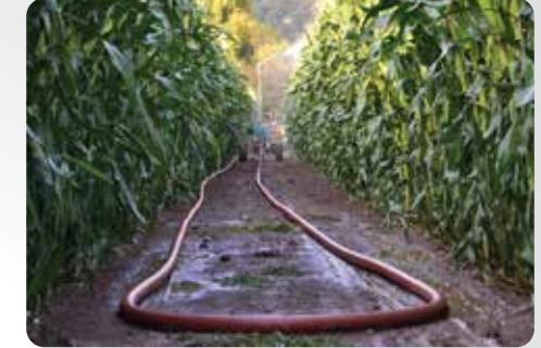
Irriforce is an irrigation machine designed for Energy Efficiency. Its cost in terms of both use and investment is lower than those of its rivals. We may call Irriforce as traveling rain gun. Thanks to water turbine and steel rope in it, it irrigates your field by dragging itself.
